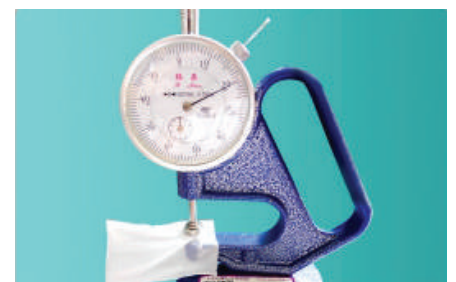
After Hydration, it does not swell up (0.205mm)
